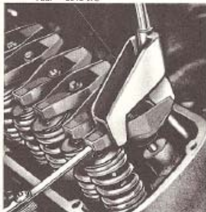
Checking valve clearance on engines with hydraulic lifters
