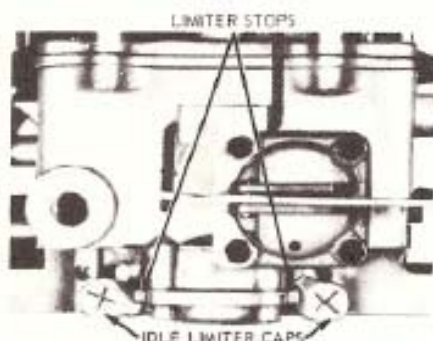
Mixture adjustment screws on the 2100 or 2150 carburetor with the limiter caps in place
