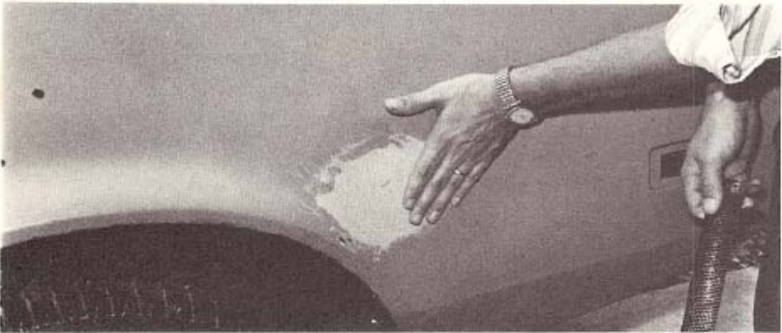
Step 8. Check frequently with the palm of your hand for high and low spots. If you wind up with low spots, you may have to apply another layer of filler
