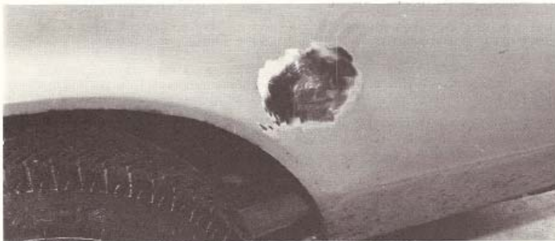
Step 3. The area should look like this when you're finished grinding
