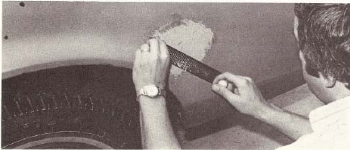
Step 7. Knock the high spots from the body filler with a body file
