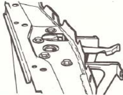
The base of the hood lock can also be repositioned slightly to give more positive lock engagement
