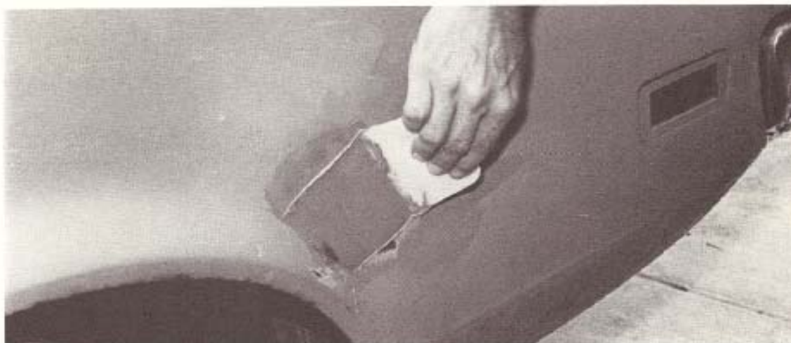
Step 5. Spread the body filler evenly over the entire area. Be sure to cover the area completely
