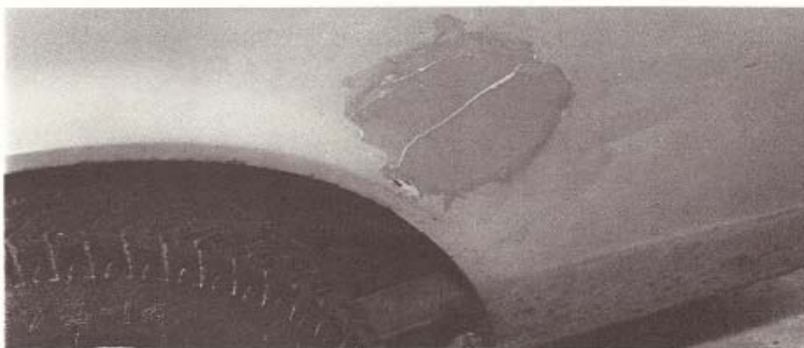
Step 6. Let the body filler dry until the surface can just be scratched with your fingernail
