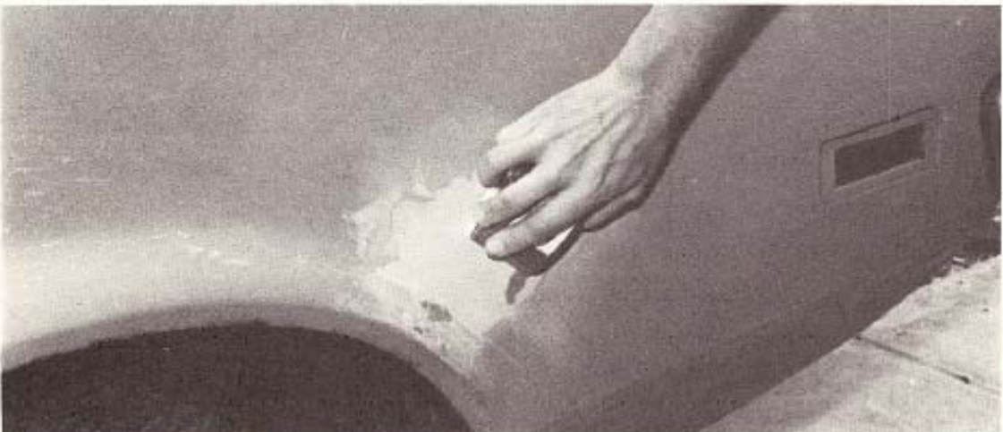
Step 9. Block sand the entire area with 320 grit paper
