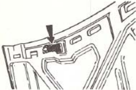
The hood pin can be adjusted for proper lock engagement
