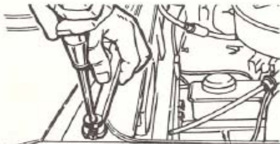
The hood is adjusted vertically by stop-screws at the front and/or rear
