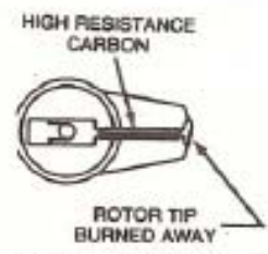
Inspect the distributor cap and rotor
