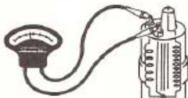
Check the coil primary resistance
